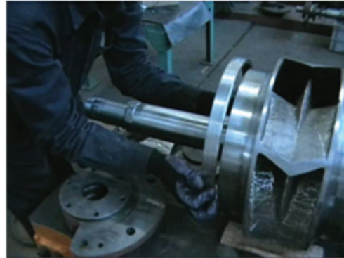
Picture 4 - Neck Ring Installation
